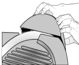
FIG 3. INSTALLING THE SHARPENER BOX
